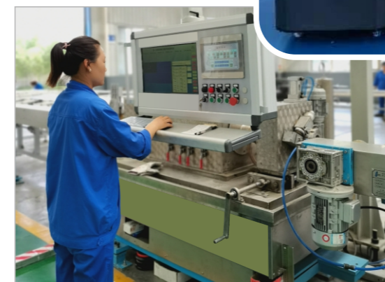
▶ SUT-DK-TB型全自动旋转头超声波探伤机 Automatic Rotating Head Ultrasonic Flaw-detecting Machine
