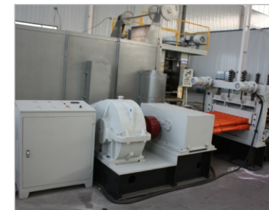
▶ 十五辊板材校平机 Fifteen-roller leveller
