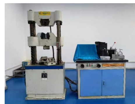
▶ 微机屏显液压万能试验机 Computer screen display hydraulic universal testing machine
