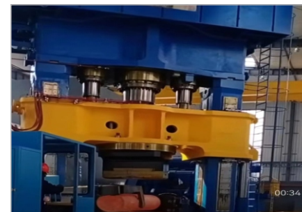
▶ 25MN快速液压锻造机 25MN fast hydraulic forging machine
