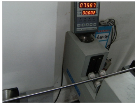
▶ 红外线测径仪 Infra-ray diameter gauge
