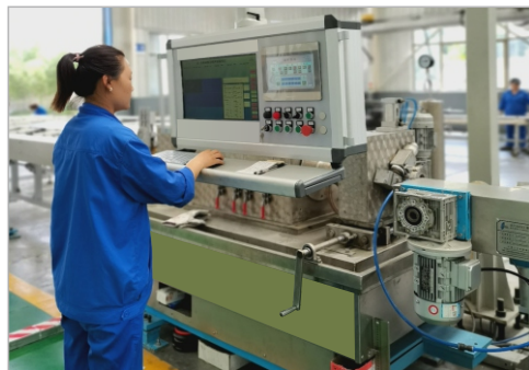
▶ SUT-DK-TB型全自动旋转头超声波探伤机 Automatic Rotating Head Ultrasonic Flaw-detecting Machine
