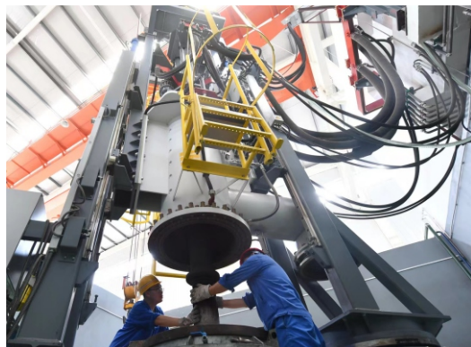
▶ 德国进口ALD真空熔炼炉 ALD vacuum melting furnace imported from Germany
