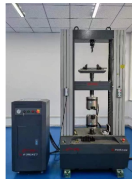
▶ 微机控制电子万能试验机 Microcomputer control electronic universal testing machine
