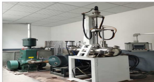
▶ 5kg 实验用VAR熔炼炉 5kg VAR melting furnace for testing
