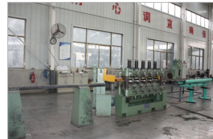
▶ 斜辊式校直机 Inclined three-roller straightening machine
